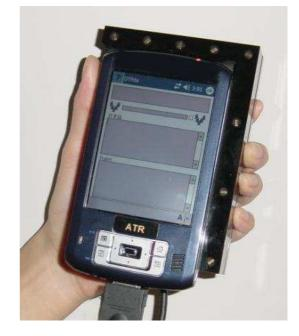
Figure 2. Mobile multi-channel speech input device with PDA terminal. Eight microphones are arranged as reverse L-shaped array.
